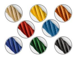
Corocord ropes with 19mm diameter or more are special 'Hercules' - type with galvanized sixstranded steel wires. Each strand is tightly wrapped with PES yarn, which is melted onto each individual strand. The ropes are highly wear-and vandalism-resistant and can be replaced at site if needed.
