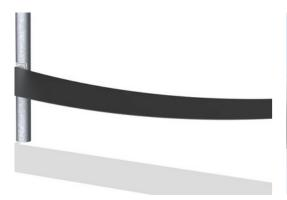
Membrane consisting of friction-proof rubberized material of conveyor belt quality with excellent UV resistance. Tested and compliant with REACH requirements for PAH. Embedded are two layers of galvanized steel wire armoring, making the membrane extremely hardwearing and vandalism resistant. Core and outer layers result in a total thickness of 10mm.
