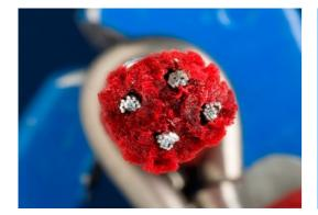
Corocord 16mm ropes of UV-stabilized PES rope strands with inner steel cable reinforcement. The polyester yarn is made from +95% post-consumer materials and is inductively melted onto each strand. The ropes are highly wear-and vandalism-resistant and can be replaced at site if needed.
