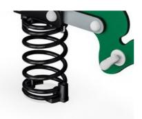
KOMPAN Springs are made of high quality spring steel according to EN10270. The springs are cleaned by phosphating before they are painted with an epoxy primer and a polyester powder coating as top finish. The springs are fixed by unique anti pinch fittings for maximum safety and long lifetime.
