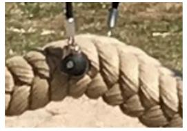
The chain/ropes are attached to the Coconut rope by KOMPAN's swivel bushings which are made of stainless steel with bronze bearings. The swivels have an outer cover which is manufactured from black PUR. The usage of side mounted swivels provides frictionless movement, eliminates fingers and feet entrapments and enlarges the standing surface on top of the rope.
