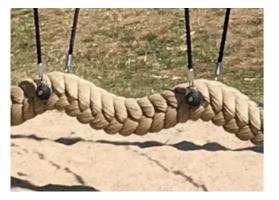
The rope of the pendulum swing is made of polypropylene (PP) rope in Coconut style with a square shape of 14x14cm. The ends of the Coconut rope are closed by steel clamps and sealed by a glued-on shrinkable tubing. The last 10cm of the rope ends are cut open to make a tassel with bumper function to fulfil global safety requirements.
