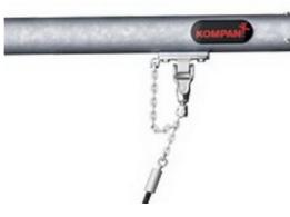
Vertical posts of hot dip galvanised steel or powder coated on pre-galvanised steel base. Swing frame end connectors and crossbeam of hot dip galvanised steel or powder coated on hot dip galvanised steel base. KOMPAN heavy duty designed swing hangers of stainless steel with anti-twist function. The hangers are attached to the cross beam on a welded bracket with two bolts, The bearings are embedded with silicone lubricant and needs no further lubrication.
