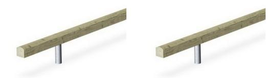
Beams are made of pine wood from sustainable European sources. The wood is pressure impregnated Class 3 with Tanalith E3475 according to EN335 (Equivalent to NTR Class AB). The steel surfaces are hot dip galvanised inside and outside with lead free zinc and with powder coated top-finish. The galvanisation has excellent corrosion resistance in outside environments and requires low maintenance.
