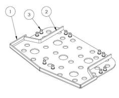
A 5 mm hot-dip galvanized carbon steel plate to the frame.
