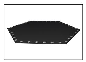
The jumping membranes are made of 6.0mm thick EP Ethylene-Propylene conveyor belt with polyester polyamide fabric carcass. Spring fixations are reinforced with steel bushings and washers on both sides. The membrane is ozone resistant and equipped with 8 center placed water drain holes.
