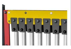
Membranes consist of friction-proof rubberised material of conveyor belt quality with excellent UV resistance which is then embedded is a fourlayered armouring made of woven polyester. The armouring and the two surface layers result in a total thickness of 9 mm.
