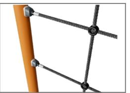
The ropes are made of UV-stabilised PES with inner steel cable reinforcement. The rope is induction treated in order to create a strong connection between steel and rope which leads to good wear resistance.
