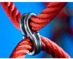
Corocord 'S' clamps are used as universal connections in Corocord products. 8mm stainless steel rods with rounded edges are pressed around the ropes with a special hydraulic press, making them the ideal connector: safe, durable and vandalism-proof, all while allowing the typical movement of rope play structures.
