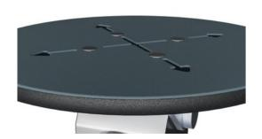
The ø414mm top plate is made from 15mm Ekogrip®, a 15mm PE plate with a 3mm toplayer of thermoplastic rubber with non-skid effect. The height is 217mm and the range of motion is +/- 90°, with a EPDM rubber stop at each end.
