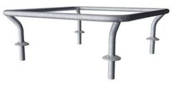
Handrail intended as grips during exercises are made of hot-dip galvanised steel ø38mm, a great diameter for a good grip and to support the wrist. The height of the handrail is 940mm from the top of the HPL plate. The distance between the rails is 900mm.
