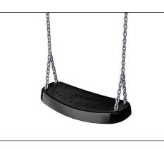
The standard seats of KOMPAN swings is engineered for maximum safety and durability. The two component seat with a PP inner core and outside rubber is produced in one operation. The seats are available with swing chains of either hot dip galvanised steel or stainless steel for all swings heights.
