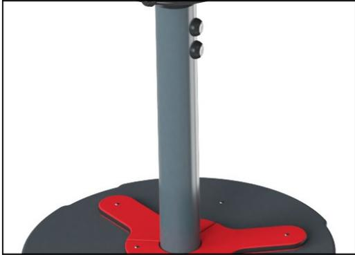
Posts are made of high quality galvanised steel with optional powder coated top finish. The galvanisation has excellent corrosion resistance in outside environments and requires low maintenance.
