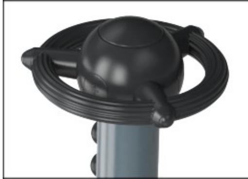
The upper round handle is made with a galvanised steel insert and covered with soft PUR rubber with grooves that ensures good handhold while rocking.
