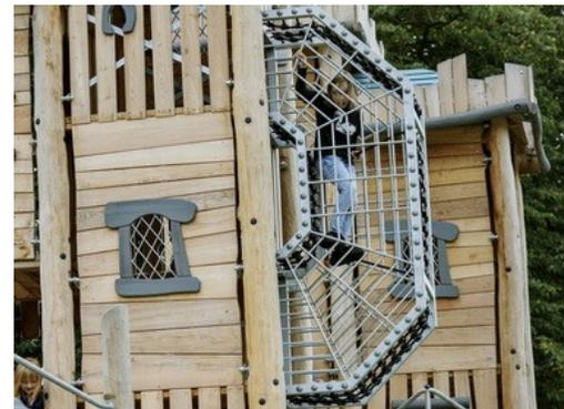
The wire frame tunnel is made of hot dip galvanised high quality steel. Corocord 16mm ropes are special 'Hercules'-type with galvanised four-stranded steel wires and a steel wire core. Each strand is tightly wrapped with PES yarn, which is melted onto each individual strand.
