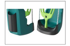
The front bumper has a solid polypropylene (PP) core with a softer outer layer of thermoplastic rubber (TPE) and an 8mm thick EPDM membrane rear bumper. The soft, shockabsorbent bumpers with nonslip surfaces make the swing seat highly safe for caretakers.
