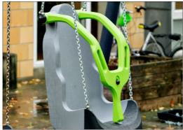
The Harness is made of molded recyclable polyethylene (PE) from 33% post-consumer materials. The Harness utilizes a stainless-steel torsion spring, which makes the Harness stay in all positions to secure easier user entry and exit. The harness lock is designed with a one-handed operation slider made from stainless steel.
