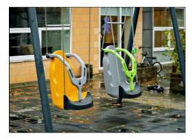
The inclusive swing seat is made of recyclable polyethylene (PE) using 33% post-consumer materials. The seat is molded in one piece and equipped with a drain hole to avoid water accumulation. The ergonomic design enables a safe and comfortable seating position.
