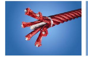
Ropes of UV-stabilized PES rope strands with inner steel cable reinforcement. The polyester yarn is made from +95% post-consumer materials and is inductively melted onto each strand. The ropes are highly wear-and vandalism-resistant and can be replaced at site if needed.
