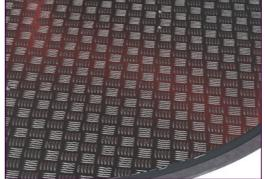
Deck plate of 3mm thick non skid aluminum or 17,8mm thick HPL plate. For warm locations KOMPAN recommends HPL deck plate as the aluminum will get hot in sunny conditions. Both deck plates ensures safe play for all users and is maintenance free.
