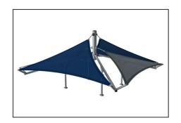
Sails of commercial 95 high-density PE knitted specially for sun-shade structures. The sails are treated with UV stabilisers to ensure longevity. The sails are supported by a hot-dip galvanised steel frame and tightened by stainless-steel devices.
