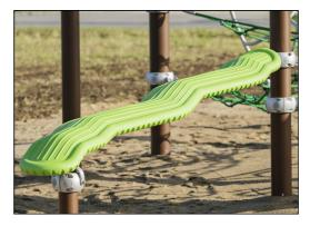
Rocking tube is made of medium density PE with excellent impact strength and usable within a large temperature span. Hollow plastic components are made of 100% recyclable PE made from 33% post-consumer materials. Molded in one piece with minimum 5mm wall thickness. The longitudinal grooves provides a slip resistant surface for safe play.
