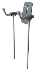
The frame of the leg lift is made from Ø38 x 2mm HDG steel tube. The support plates are made from 15mm Ekogrip®, a 15 mm PE plate with a 3 mm top-layer of thermoplastic rubber with non-skid effect. The arm supports are 110 x 195mm, 580mm apart, and 1315mm above ground. The back support is 335 x 500mm. The opening in the back is 30 x 350mm.
