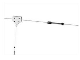
The high-quality steel cable with a diameter of 12mm is designed for heavy usage of the cableway for many years. The starting point is indicated by a knob. At the stop point, there is a uniquely designed spring device, ensuring a softer stop of the puller.
