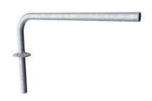
Handrail intended as grips during exercises are made of hot-dip galvanized steel ø38mm, a great diameter for a good grip and to support the wrist. The height of the handrail is 940mm from the top of the HPL plate. The distance between the rails is 900mm.
