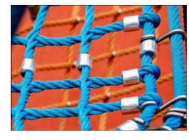
The aluminium swages of the net are double conical with rounded ends and are as small as safety allows. The overall net design aims at keeping metal parts within the net to an absolute minimum, both in size and number, in order to provide the best possible rope climbing experience.
