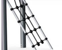
Nets and ropes are made of UV-stabilized PA with inner steel cable reinforcement. The rope is induction treated in order to create a strong connection between steel and rope which leads to good wear resistance.
