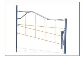
ELEMENTS ropes have six-stranded steel wires and a steel wire core. Each strand is tightly wrapped with PES yarn, which is melted onto each individual strand. After initial friction has removed the surface fibres, a harder PES coating remains to protect each strand, making the ropes highly wear and vandalism resistant.
