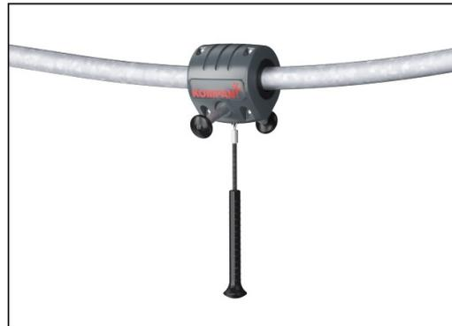
The hang-on puller is designed with a welded steel core and covered with low-density PE housing. The two hot dip galvanised steel handles are angled to provide best possible ergonomic while gliding. The wheels of the puller are made of low noise TPU and installed with sealed ball bearings.
