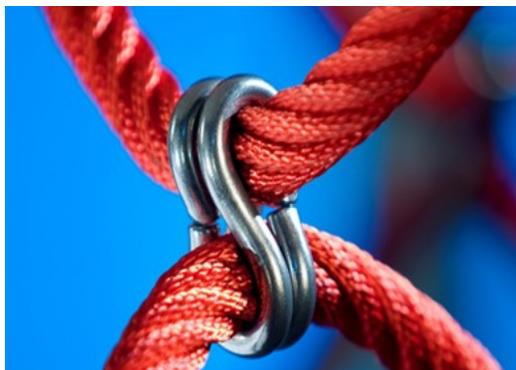
Corocord 'S' clamps are used as universal connections in Corocord products. 8mm stainless steel rods with rounded edges are pressed around the ropes with a special hydraulic press, making them the ideal connector: safe, durable and vandalism-proof, all while allowing the typical movement of rope climbing structures.
