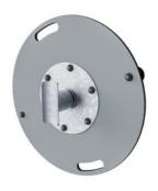
The bearing house is made from hot dip galvanised steel. The bearing shaft is made from stainless steel AlSI304. The bearing itself is made from Polyoxymethylene (POM), an engineering thermoplastic with a high stiffness, low friction, and excellent dimensional stability.
