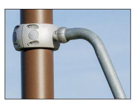
Colored steel components have a base of hot dip galvanization and a powder coated top finish. This provides an ultimate corrosion resistance in all climates around the world. Other steel surfaces are hot dip galvanized inside and outside with lead free zinc.
