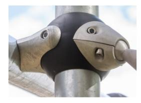
The unique designed GALAXY connection ball is made with an inner circular core of aluminium surrounded by a shell of hard PP with a outer layer of soft TPV rubber. Flexible lead free aluminium connectors allow for installation in variable angles.
