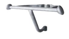
The support handle is 530mm wide. The handle is 1050mm above ground level, and 1140mm above the jumper membrane. The handle is made from a 32mm diameter HDG bar.
