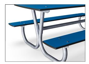
All boards are made of High Pressure Laminate HPL with a .7 in. thickness according to EN 438-6 and has a nonskid surface texture. The multilayer construction makes the boards durable and suited for outdoor use, with a high resistance to impacts, scratches, fire, water and humidity, as well as high UV stability.
