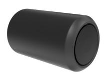
The rotating rollers are Ø 110mm and made from PUR (Polyurethane Rubber, compact foam). The rollers have a steel insert that is electro galvanized. They provide support and ensure a comfortable position. All Steel components are made from carbon steel, with a hot-dip galvanized surface according to ISO1461, and a powder coating corrosion class C3 according to ISO12944-2. Lead content for surfaces is below 90ppm, and below 100ppm for base material.
