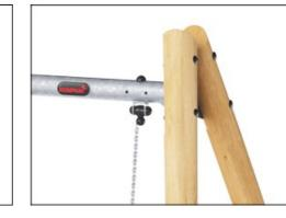
The swing hangers are made of high quality UVstabalised nylon (PA6) housing with integrated lifetime sealed ball bearings. The height adjustable chains are fixed by a stainless steel hook with theft proof snake-eye bolt in a turn able anti twist housing. All seats with two chain fixation are available with either standard or anti-wrap suspension.
