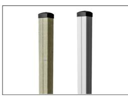
The main tower posts are available in two types of material: European pine wood posts, pressure impregnated Class 3 with Tanalith E3475 according to EN335 (Equivalent to NTR Class AB). Aluminum post t=2mm with anodized surface treatment. Base material EN AW-6060 T66.
