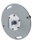
The bearing house is made from hot-dip galvanised steel. The bearing shaft is made from stainless steel AISI304. The bearing itself is made from polyoxymethylene (POM), an engineering thermoplastic with high stiffness, low friction, and excellent dimensional stability.
