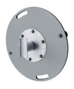
The bearing house is made from hot-dip galvanised steel. The bearing shaft is made from stainless steel AISI304. The bearing itself is made from polyoxymethylene (POM), an engineering thermoplastic with high stiffness, low friction, and excellent dimensional stability.
