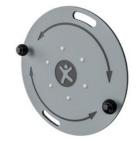
The ø800x19mm wheel is manufactured from HDPE EcoCore<sup>™</sup>, which is a highly durable, eco-friendly material, that is recyclable after use and produced from 100% recycled material. The core has a thickness of 15mm and is representing 80% of the total material.
