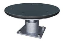
The bearings used in the twist are slide bearings. These are made from extremely strong polyoxymethylene which is low wearing, highly mechanical, moisture absorbant and provides high abrasion resistance. The ø414mm top plate is made from 15mm Ekogrip®, a 15mm PE plate with a 3mm toplayer of thermoplastic rubber with non-skid effect. The height is 217mm and the range of motion is  $+/-90^{\circ}$ , with a EPDM rubber stop at each end.
