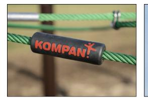
Ropes are made of UV-stabilized PES rope strands with inner steel cable reinforcement. The polyester wrapping is inductively melted onto each strand to ensure excellent wear and tear resistance. Colored steel components have a base of hot dip galvanization and a powder coated top finish. This provides an ultimate corrosion resistance in all climates around the world. Other steel surfaces are hot dip galvanized inside and outside with lead free zinc.
