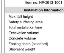
0 cm 14.9 m<sup>2</sup> 4.8 0.38 m<sup>3</sup>  $0.00 \text{ m}^3$ Footing depth (standard) 100 cm 168 kg In-ground Anchoring options Surface **Warranty Information**
