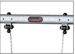
The swing hangers are made of high quality UV-stabalised nylon (PA6) housing with integrated lifetime sealed ball bearings. The height adjustable chains are fixed by a stainless steel hook with theft proof snake-eye bolt in a turn able anti twist housing. All seats with two chain fixation are available with either standard or anti-wrap suspension.
