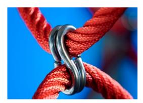
Corocord 'S' clamps are used as universal connections in Corocord products. 8mm stainless steel rods with rounded edges are pressed around the ropes with a special hydraulic press, making them the ideal connector: safe, durable and vandalism-proof, all while allowing the typical movement of rope play structures.
