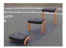
The support frame is ø48.3 x 4mm, carbon steel, with a hot-dip galvanised surface according to ISO1461, and a powder coating corrosion class C3 according to ISO12944-2. Lead content for surfaces are below 90ppm.
