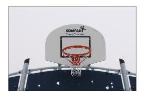
The basketball hoop is made from hot dipped galvanised steel with a powder coated finish and a backboard made from +95% PCR HDPE. The net is made from 100% nylon, with a circumference of ~Ø30cm at the bottom and ~Ø50cm at the top. The net can also be supplied with steel reinforced PA net or steel chains.
