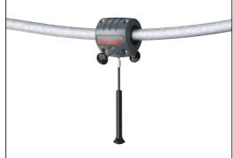
The hang-on puller is designed with at welded steel core and covered with low-density PE housing. The two hot dip galvanised steel handles are angled to provide best possible ergonomic while gliding. The wheels of the puller are made of low noise TPU and installed with sealed ball bearings.
