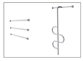
Pipe ladder bars are hot dip galvanised inside and outside with lead free zinc. The galvanisation has excellent corrosion resistance in outside environments and requires low maintenance.
