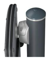
The connectors are made of die-cast aluminum specially alloyed for outdoor environments and with a lead content below 100ppm. The connectors are attached to the posts by stainless steel screws and well protected against corrosion by special designed zinc washers. Extremely strong and no change of corrosion.
