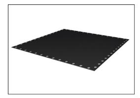
The jumping membranes are made of 6,0mm thick EP Ethylene-Propylene conveyor belt with polyester polyamide fabric carcass. Spring fixations are reinforced with steel bushings and washers on both sides. The membrane is ozone resistant and equipped with 8 center placed water drain holes.
