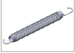
All 52 springs are made of stainless steel to ensure durability and excellent corrosion resistance. The steel wire is 3,2 mm thick and the last five windings are cone shaped to ensure long lifetime of the jumper.
