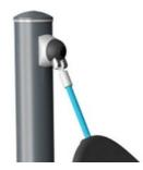
KOMPAN's unique swivel suspensions allow for both swinging and rocking movement when children play on the hammock. The inside housing is made of stainless steel, and both the bushing and bearing rod is made from brass alloy. The outside cover is made of soft TPV rubber, and the entire swivel is attached to the steel post by an aluminium connector.
