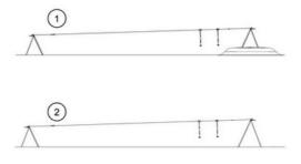
KOMPAN cableways are available for flat or natural sloped surroundings and for surface or in-ground installation. Further the cableways can be supplied with one or two cables for children to ride together in friendly competition. For flat surroundings a starting mound or platform is needed to use the cableway.
